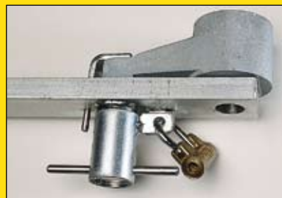
The manual release mechanism is either a threaded pin for gates or a quick release for doors. Both types are lockable. The drive arm linkage protects the gearbox in the event of accidental collision damage.
