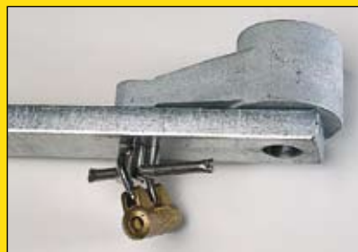
The manual release mechanism is either a threaded pin for gates or a quick release for doors. Both types are lockable. The drive arm linkage protects the gearbox in the event of accidental collision damage.
