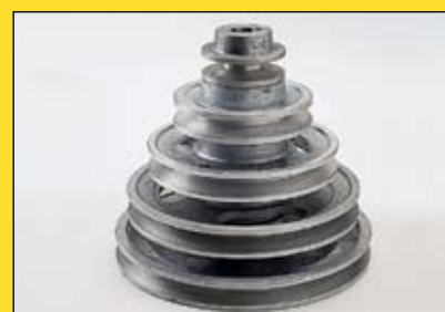
The speed and torque are easily adjusted by changing the drive pulleys.
