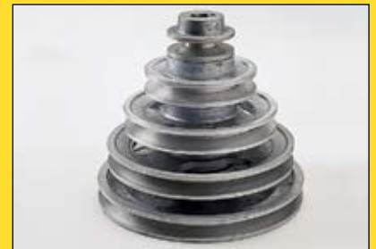
The speed and torque are easily adjusted by changing the drive pulleys.
